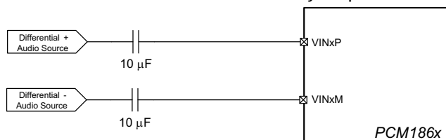
Figure 56. Analog Input Circuit for Differential Input Applications
